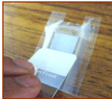
Figure 7. Coating the transparent glass plate with \text{TiO}_2 paste
