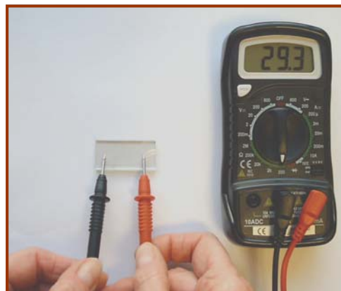
Figure 4. A multimeter being used to determine the conducting side of a transparent glass plate
