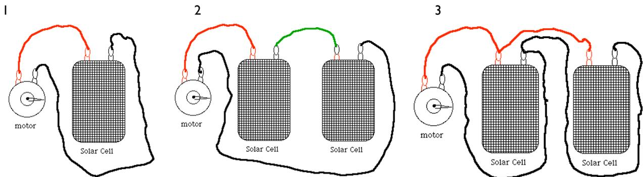
1. A solar cell is connected to a motor with clip leads.
