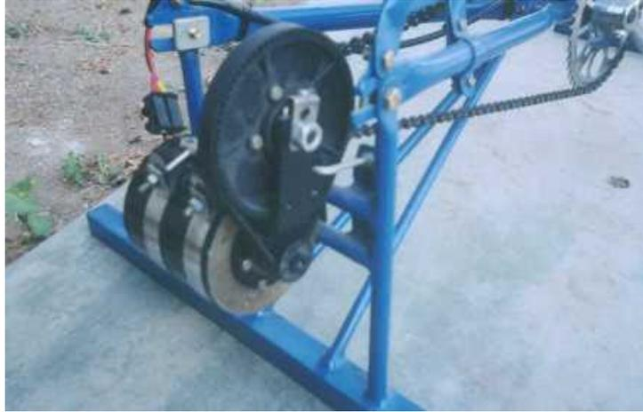
The above photo shows a close up of the generator and drive pulley assembly, flywheel was removed for better clarity:
